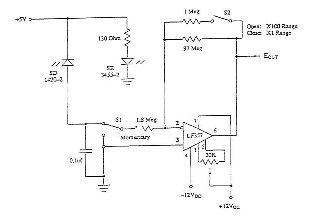
Figure 13 – Tape light transmission test circuit
