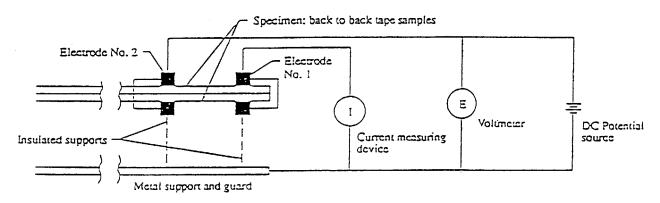
Figure 4 – Tape resistance measument circuit
