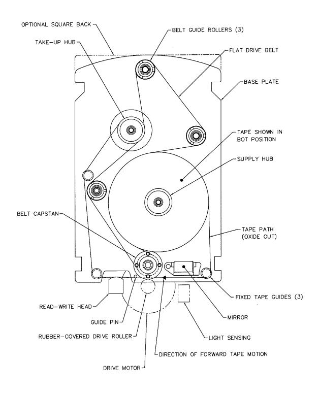
FIG. 1 - CARTRIDGE CONFIGURATION
