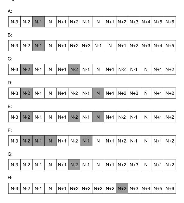
Figure 9.11 Examples of Possible Format Layout Variations Due to Block Rewrite Operations (Shaded Denotes a Bad Block, N Denotes a Physical Block Address)
