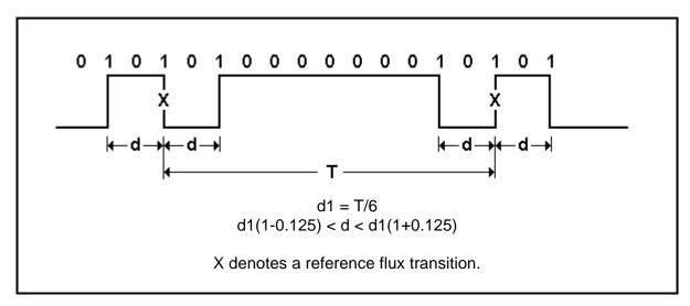
Figure 5.3 Test Pattern for Instantaneous Flux Transition Spacing Test.
