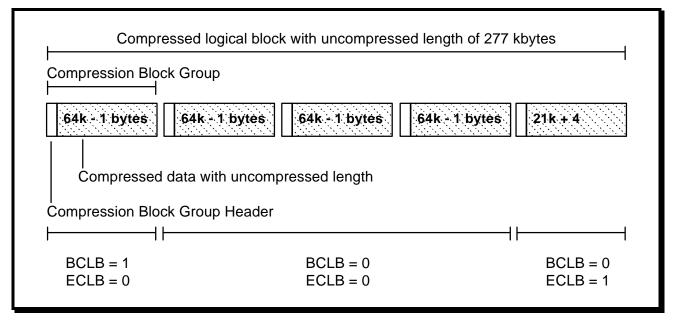
Figure 10.1 Logical block spanning multiple Compression Block Group
