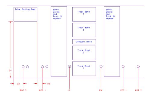
Figure 6.1 General Tape Layout and Dimensions for DWA
